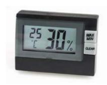
Electronic precision instrument for measuring the temperature, humidity and the highest and lowest values of both (MAX-MIN function).
